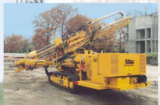
Mobile deep drill rigs, Hütte & Co.
